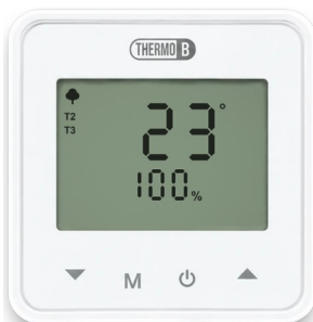
2 – outdoor temperature and valve position
