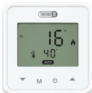
1 – main: S1 temperature, setpoint, mode
